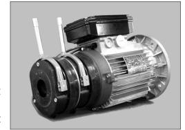
Rectifiers are provided with an overvoltage protection device and with an EMC filter. It's possible to have two types of wirings connection to the rectifier for each brake, in relation to the intervention time required.
